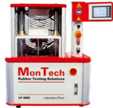
LP 3000 - 200kN Medium size benchtop hydraulic laboratory press
