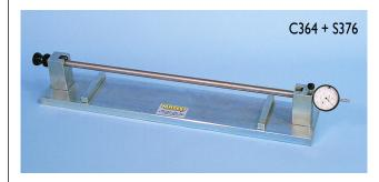
DETERMINATION OF RESTRAINED EXPANSION OF CON-CRETE AND MORTAR CONTAINING THE EXPANSIVE AGENT STANDARDS: UNI 8148, 8147 - EN 1367-4
