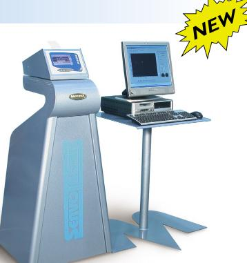
Servotronic C104 connected to a PC H009-01 with "Servonet" Licence C123 for the managing and the remote control of the test throughout all the phases.
