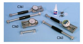
**Strain gauges**, identical to above (C360÷C361), but equipped with a "**digital gauge**", battery feeded, with reading values in mm (sens. 0,001 mm) and in inch (sens. 0,0001"). Complete with battery and RS 232 connector to PC.
