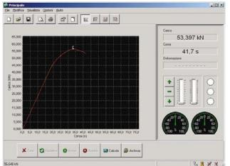
C109-12 Graphic example on Tensile Splitting Test.
