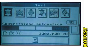
Menu of a test starting with automatic execution.
