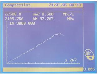
8 • Graphic representation of the load/time behaviour on the test effected.
