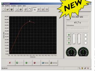
C109-12 Graphic example on Tensile Splitting Test.
