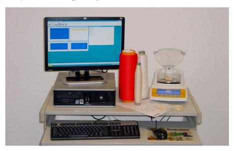
The TEXCOUNT TT support all count systems, such as Nm, tex, ktex, Nec, New etc. The test data provided by the TEXCOUNT software are:
