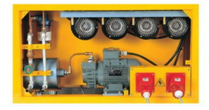
These extruders are also equipped with a built in high capacity vane-type vaccum pump. Including large inlet filters, as well as a vaccum dial gauge and release valve mounted on the top of the extruder barrel behind the vent opening.
