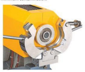
Extruder head with chromed C-Clamp, equipped with two isolated handles and a single clamping screw for easy operation. A breaker plate with slot for inserting of screens is situated at the barrel flange and can be easily accessed when the flange is opened.
