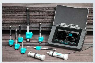
The Equotip 550 Portable Rockwell is a static hardness measurement solution which is highly appreciated for applications on thin or light samples. Furthermore, it can be used on almost all materials without special adjustments, which also makes it popular to use as a reference method for other measurement principles. A wide variety of accessories makes it very versatile.
