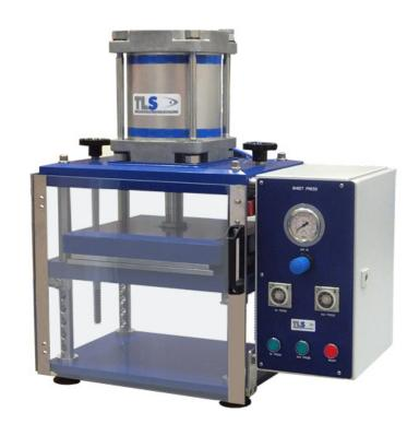
The set consists of blotting dry, drying wet, wet paper sheet and plate drying, repeated several times. Over the last plate drying a dry blotter is placed the stack of sheets in the press is placed and operated this, until an effective pressure of 400 ± 10 kPa in 20 ± 10 seconds. this pressure is maintained for a time of 5 minutes, and after the same, the pressure is lowered and the stack of sheets is removed from the press.
