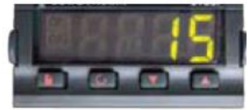
Over-temperature limit controller
