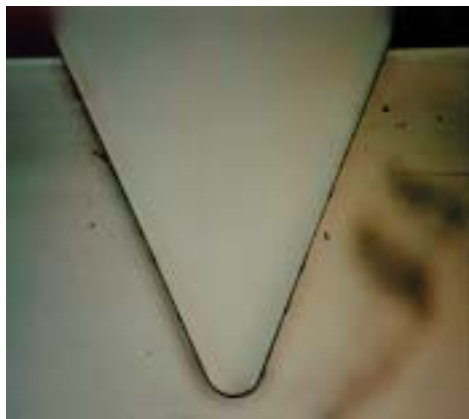
Detail of a notch obtained on ABS specimen using Automatic Notchvis. (The quality of the notch is evident)
