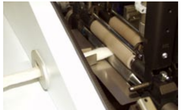
The drafting system components originate from a draw frame. The top rolls are pneumatically loaded.
