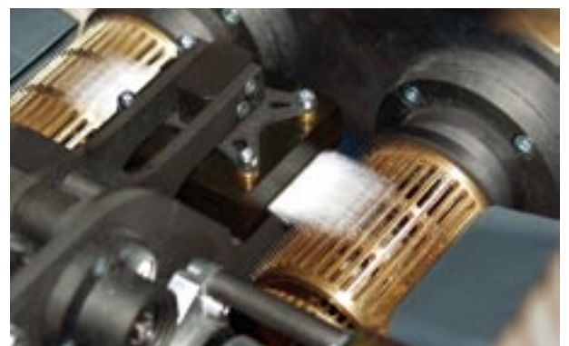
Two needle rolls with inside suction remove the loose fibres on both sides of the fibre tuft.
