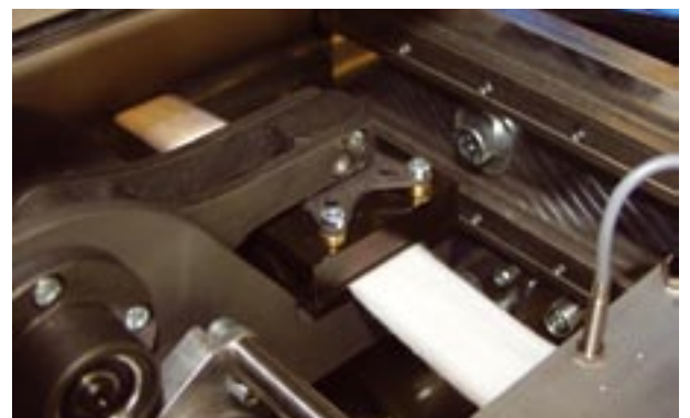
A solid clamp ensures precise fixing of the fibres.
