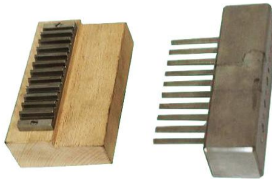
Rack and Comb device to glue the crest of the sample of corrugated paper to adhesive tape
