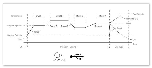
· Advanced functions include 8-segment Ramp/Dwell, USB interface, and Analog DC output capability
