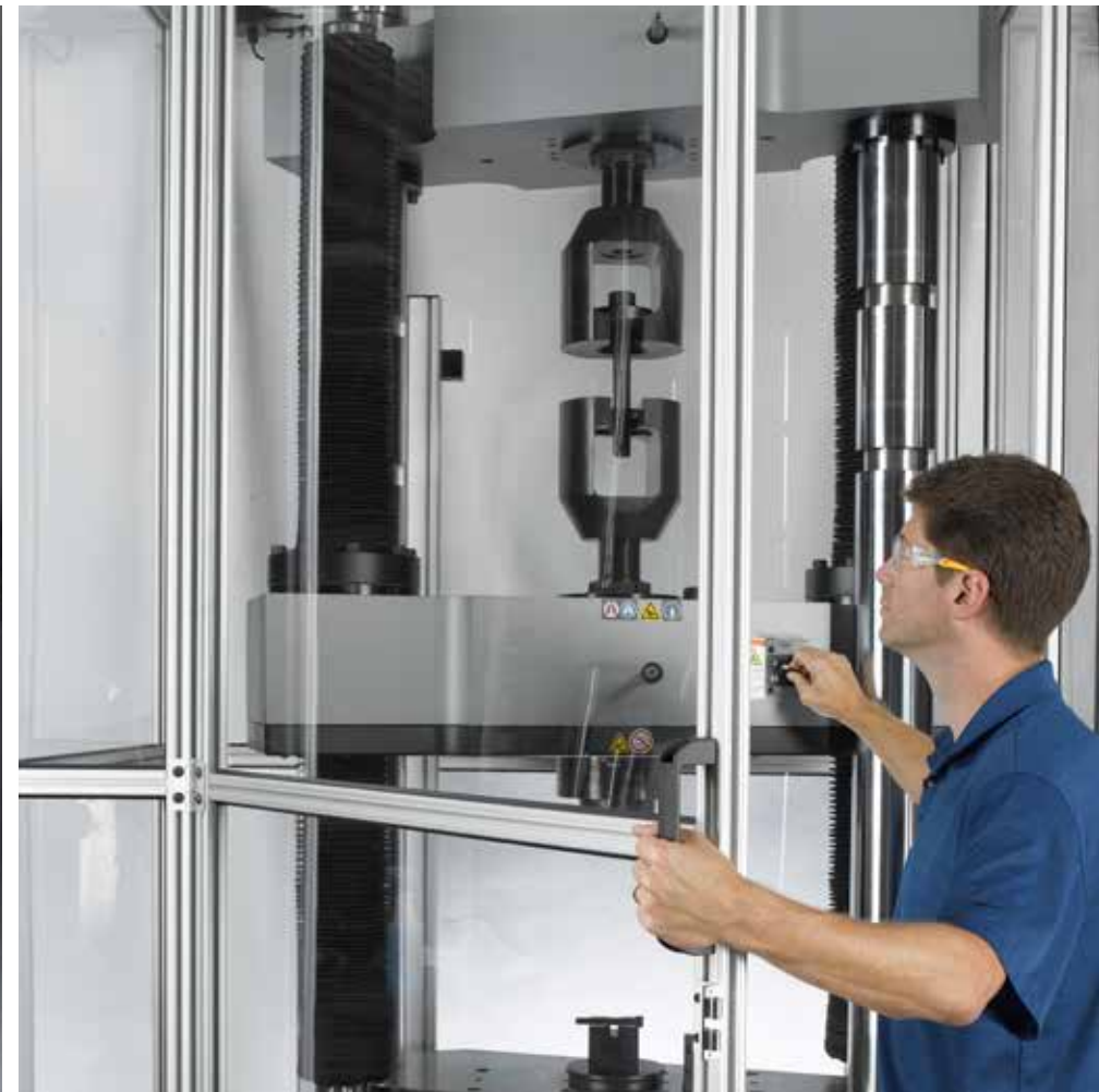
Interlocked Enclosure Prevents Operator from Entering the Test Space During Testing
