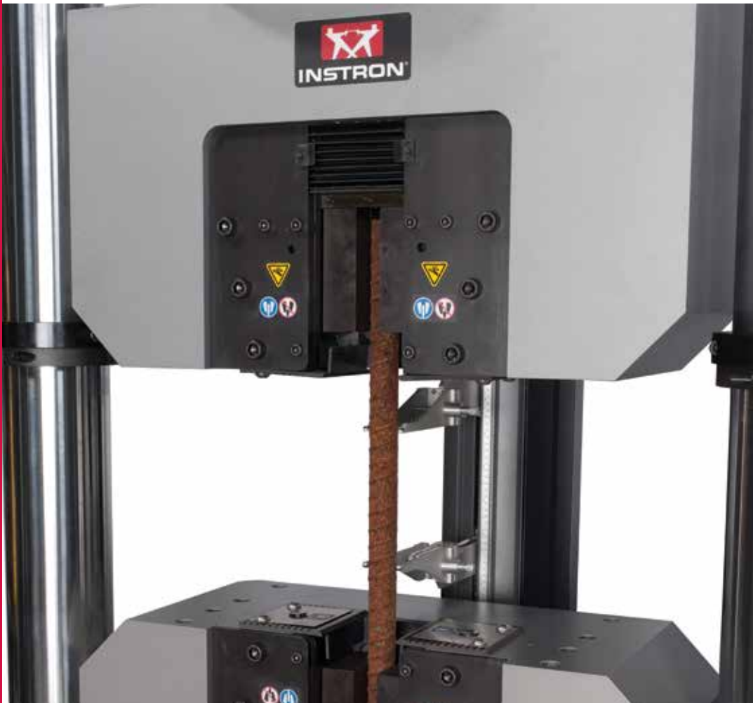
1500 kN Hydraulic Wedge Grips with AutoX Extensometer
