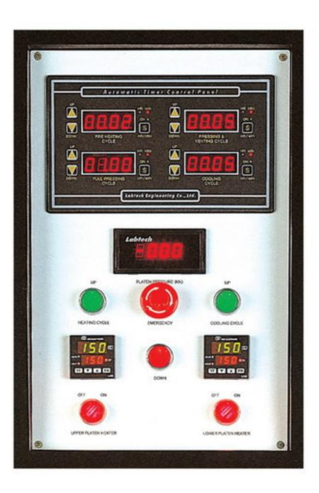
The standard **Scientific** press version is equipped with a custom made Automtic Timer Control Panel containing four adjustable timers which will automatically control all the functions, ie. preheating, pressing, venting and cooling.
