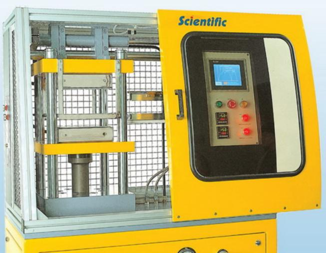
The presses are built up on sturdy welded tubular steel frames, which are totally self-supporting.
