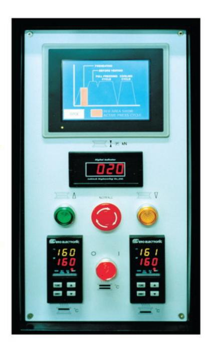
Temperature control (heating and optional watercooling) of the heating platens are regulated with two individual programmable electronic PID controller, via Electronic Proportional Relays, and thermocouples positioned near the steel surface of the platens. Each bank of heater cartridges can be individually turned on and off with switches on the control panel.
