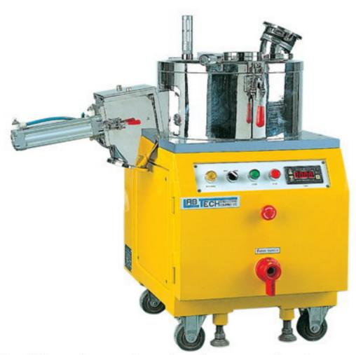
The lid to the cooler mixer is opened and swung back wards by releasing the quick lock handles to the discharge, as well as to the bowl.
