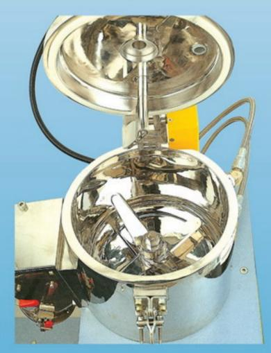
Mixer bowl lid with adjustable deflector, filter for evacuation of over pressure, as well as small lid in the center for pouring in additives even when mixer is running.
