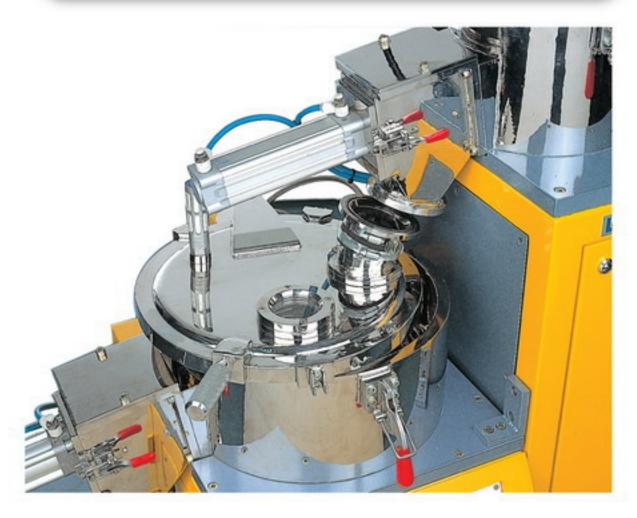
The cooler mixer, which is a separate unit on casters, can easily be attached to the high-speed mixer. It is connected to the discharge valve of the high-speed mixer with quick locks and further there are two more connecting bolts, which will attach to the body of the high-speed mixer. The electrical connections between the cooler mixer and the high-speed mixer are made from supplied cables, which plugs into the receptacles on the High-Speed mixer.
