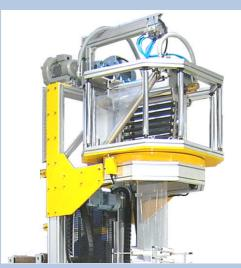
3-layer Film Blowing line, featuring three 30 mm, 30 L/D single screw extruders with film tower LF-400 CO-EX equipped with Oscillating Nip-Gap, edge cutters and electronic film web guiding system. The line has two surface windup systems for simultaneously windup of upper and lower film layer after splitting. Film tower is equipped with a motorized height adjustment where the oscillating Nip-Roller system can be raised to a height of 3.5 meter.
