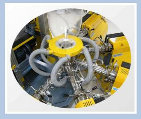
5-layers Co-Ex line featuring 5 units 20 mm, 30 L/D Single screw extruders connected to a 5-layer pancake die, with die lip diameter of 100 mm. The film tower is of type LF600 CO-EX a width of 600 mm.
