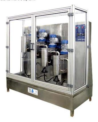
A green lamp shows that the agitation is in progress. During this time the drainage cups are furnished with weighed and marked filter papers. After the test (20 minutes according to TAPPI, 15 minutes according to SCAN) the stirrers will stop automatically and the green lamp of agitation goes out. Now shut off the water and as soon as the overflow from the last tank has nearly ceased, press the ON button of Vacuum for drainage after the completion of the agitation period.
