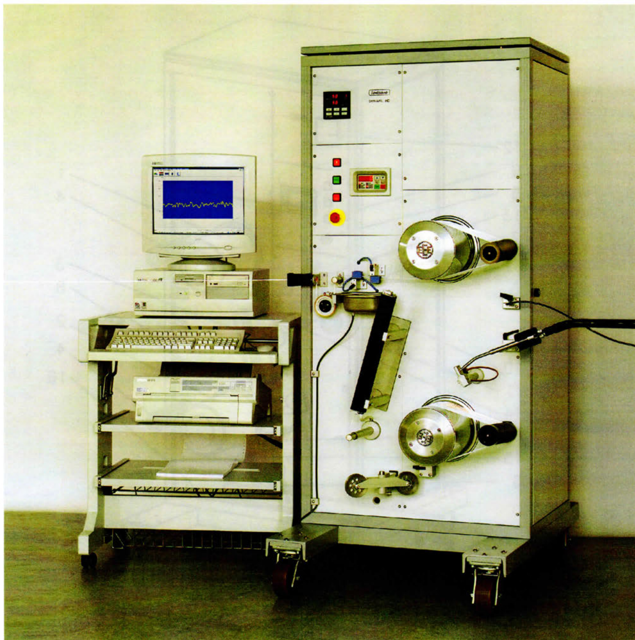
Draw force tester for coarse filament yarn and fibre tow DYNAFIL HD
