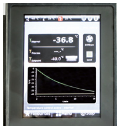
Sample temperature recording by optional immersion probe
