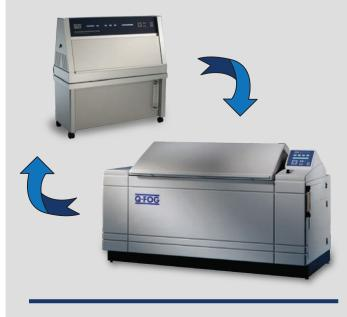
Alternating QUV exposure and Q-FOG cyclic corrosion testing can improve correlation for some materials.
