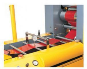
The practical windup unit is equipped with a pneumatic clamping mechanism that will grab the windup bobbin, activated by a selector switch on the side.
