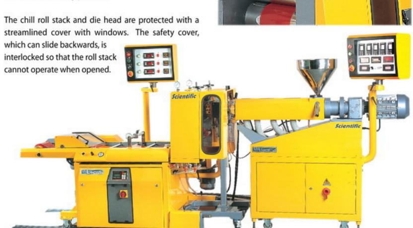
The extruder is our single screw 25 mm, 30 L/D version, which is described in details on page 21-23. The screw configuration is either plain for general QC purpose or with Maddock and screw tip mixing section for optimun mixing and blending properties. The chill roll line can also be supplied with our vented extruder version.
