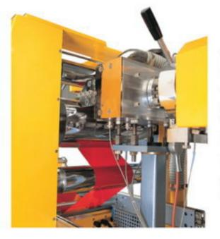
The extruder control panel is also equiped with a selector switch for Manual and Automatic mode. Thus, the extruder can also be made to run manually where the screw RPM will determine the flow of the resin to the die.
