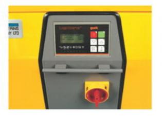
The high efficiency water heater, and chiller unit is built in to the sub cabinet. It supplies tempered water to all the rolls, regulated by valves. Optionally, more tempering units can be added for individual regulation of each roll.
