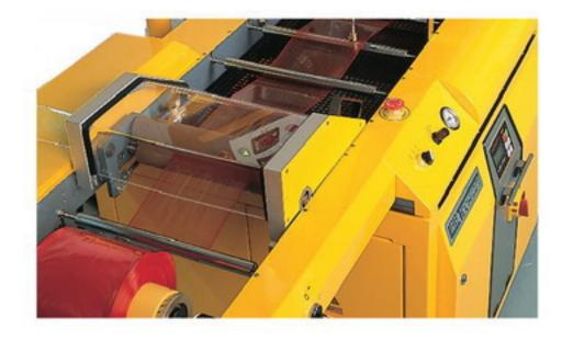
The rubber nip roll are completely protected under a Plexiglas cover, which gives full protection so that the rolls can not be touched while the machine is running.
