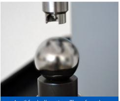
Anvil for ball testing. Therefore the indenter needs to perfectly align with the center of the anvil. Part No - 900001371
