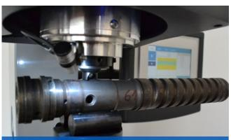
Cylindron Anvil for cylindrical parts from 50mm to 203mm in diameter. Part No. - 900007147
