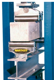
Flexure on concrete
