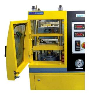
Compact fully motorized hydraulic laboratory press with modern and pleasing design. Supplied as standard with two sets of platens where the upper set has electrical heating and the lower set water cooling. Press platens are built in completely in a safety chamber with an interlocked swing open door.
