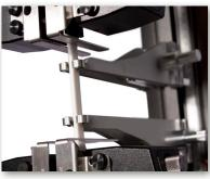
Plastic Tensile Test with AutoX750 on an Electromechanical Frame
