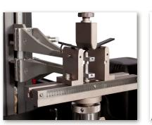
Using the AutoX750 to Measure Flexural Strain
