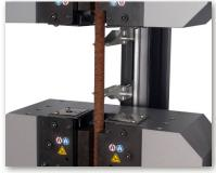
Rebar Test with AutoX750 on a 1500KPX Hydraulic Frame
