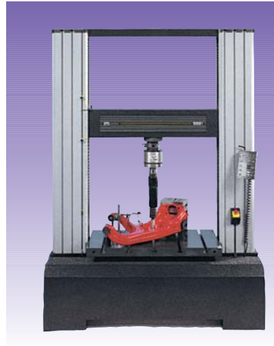
▲ Extra wide frame ideal for testing large components
