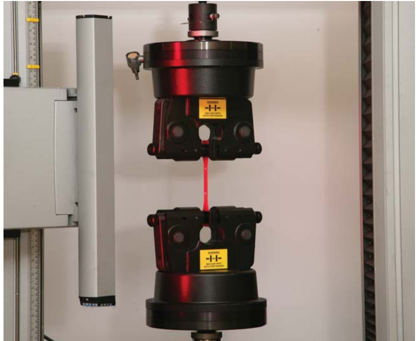
▲ Instron's Advanced Video Extensometer (AVE) is fully integrated with 5800 Series Systems.
