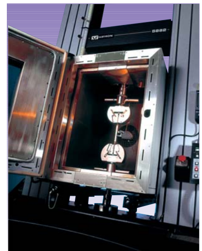
▲ Environmental chamber for elevated or low temperature testing
