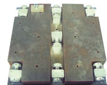
Slip table base with hydrostatic bearings
