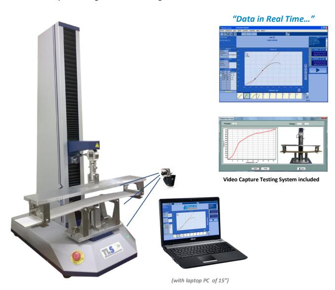
The Bending Stiffness is the ratio between the bending moment applied to a standard sample according to ISO 5628 and the deflection within the elastic area.
