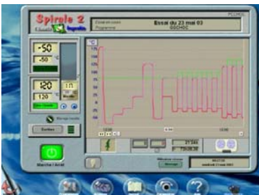
The control panel allows the access to set points, parameters and other software functions
