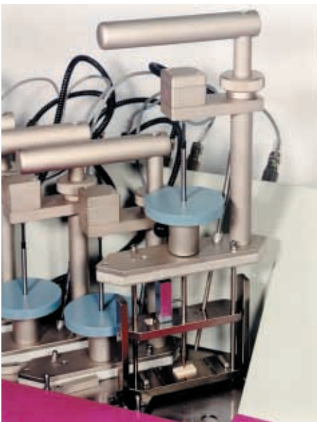
VICAT test station
