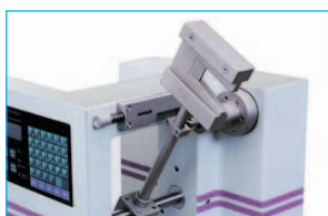
Hammer for Charpy impact tests
