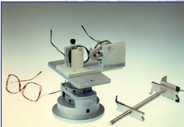
Impact test on finished products with interchangeable special striker
