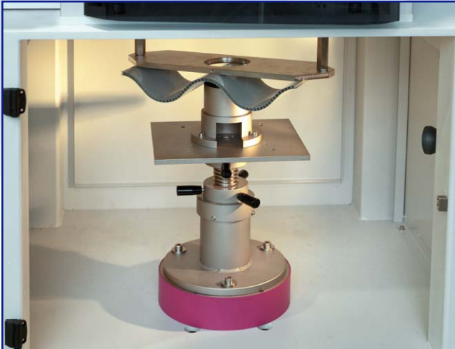
Adjustable height support and pneumatic clamping plate for pipes or similar finished products
