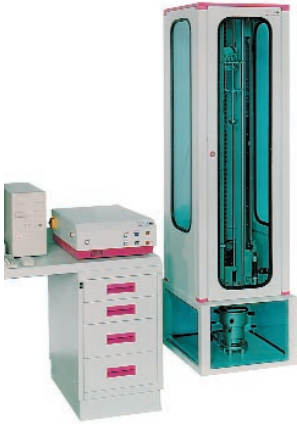
Basic apparatus code 6990.000 with control cabinet for non instrumented impact tests
