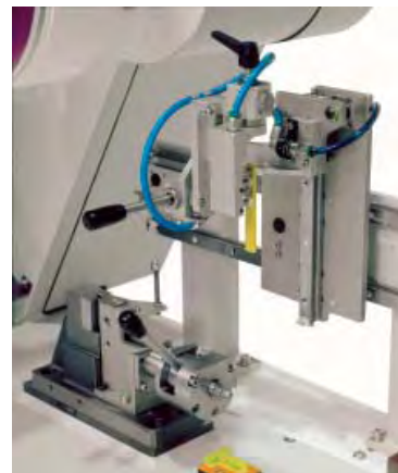
Details of Izod Specimen Positioning in Vice Using Suction Cups and Rotating Lever. Shown with Izod Vice 6956.026, also Valid for Pneumatic Foot Closure vices 7250.010 and 7250.011
