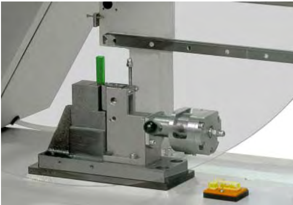
Izod vice with lever closure complete with adapters
