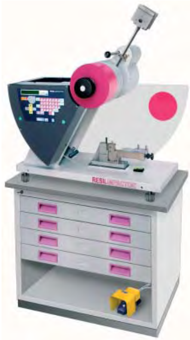
Resil Impactor 25 J Shown with Peumatic, Foot Closure Vice for Izod Specimens - 7250.010
