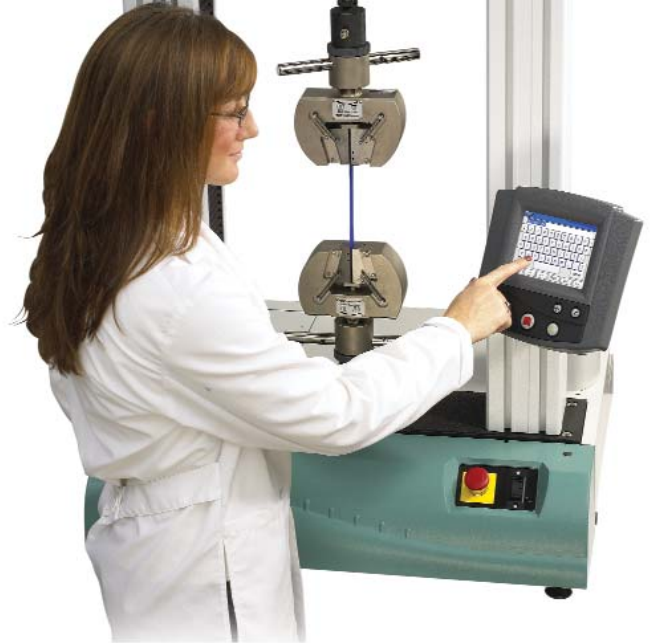
▲ The operator panel includes a software alpha-numeric keypad to enter sample ID, comments, and control parameters.
