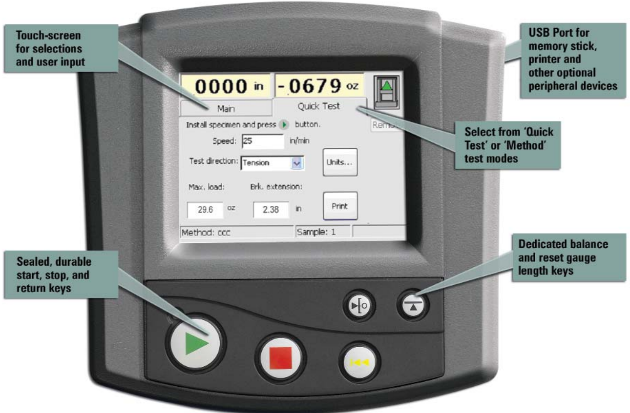
▲ The operator panel includes a software alpha-numeric keypad to enter sample ID, comments, and control parameters.
