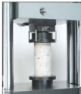
▲ External fixtures and adapters can be added to perform bend, flexure, shear and compression tests on a variety of specimens including rebar (left), concrete (center) and soil samples (right).
