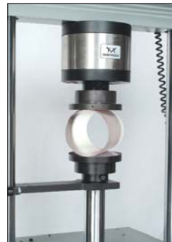
▲ Compression platens can be added to test a variety of materials and components.
