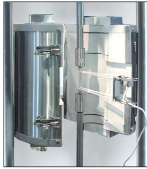
▲ Furnaces and mounting hardware can be added to test materials at elevated temperatures.
