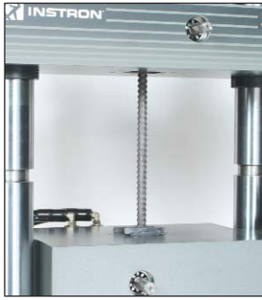
▲ In-head grips are available in V-slot or flat faces for testing samples such as bar, plate, tube, pipe, sheet and wire.
