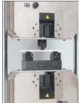
▲ Bend fixtures can be mounted to compression platens or to large tension grips.
