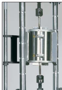
▲ Furnace and mounting hardware can be added to test materials at elevated temperatures.
