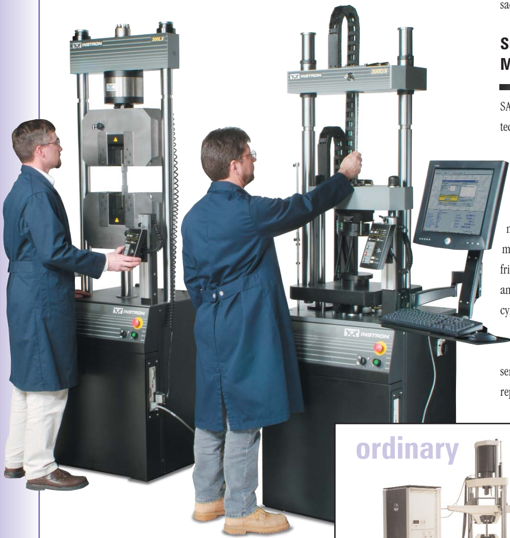
▲ 300LX frame configured for metals testing (left). 300DX frame configured for stranded wire testing (right).
