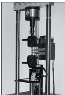
▲ Easily accessible test space is ideal for automatic extensometers.
