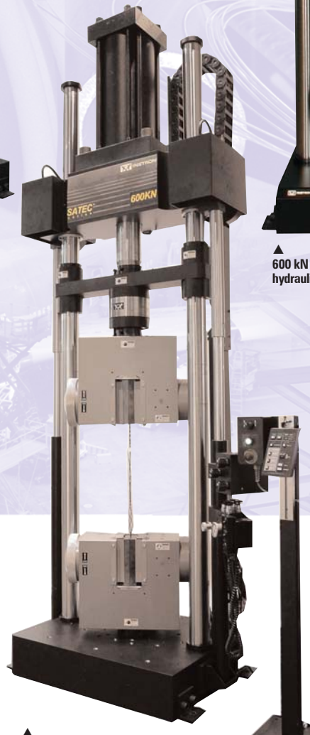
▲ 600 kN (135,000 lbf) capacity frame with single, hydraulic, side-acting grips for tensile testing of stranded wire.
