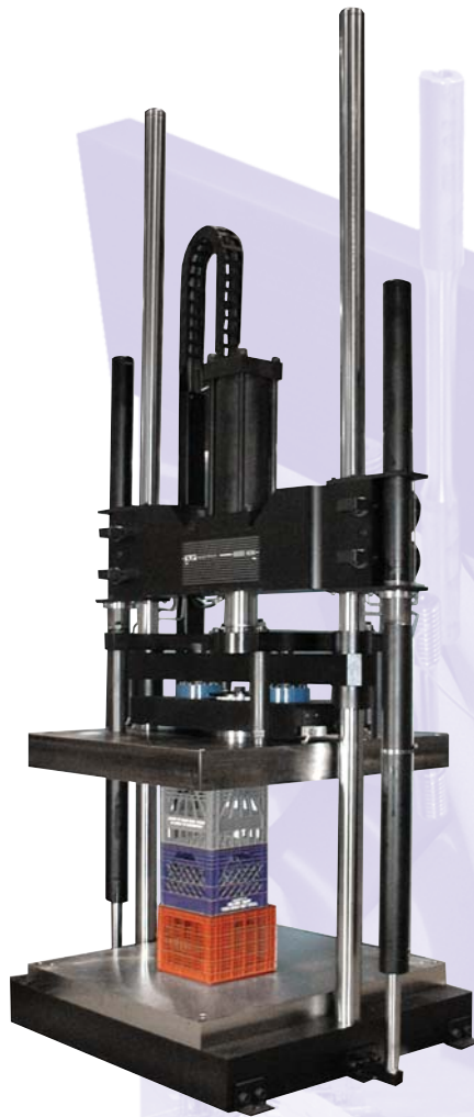
▲ Custom 600 kN (135,000 lbf) capacity frame for compression testing of plastic crates.
