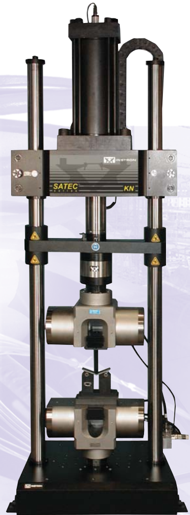
▲ 600 kN (135,000 lbf) capacity frame with hydraulic grips and guided bend test fixture.
