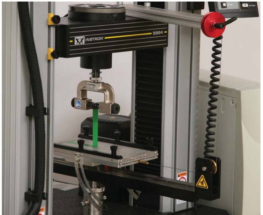
▲ 5800 Series high-speed data capture and bandwidth provide more detail in peel test results.
