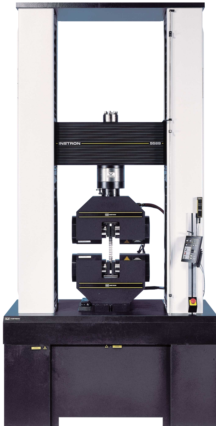
▲ Optional adapters allow secondary load strings of lower capacity fixturing without the need of removing large grips from test area
