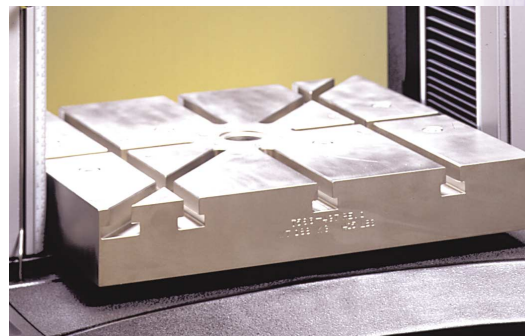
▲ T-slot table for the hard to hold down large component testing
