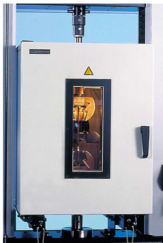
▲ 3119 Series chamber for non-ambient temperature testing
