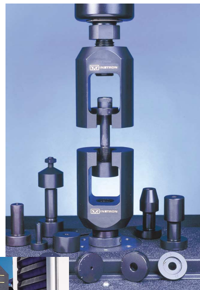
▲ Fastener tensile loading
