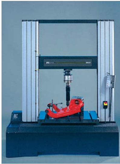
▲ Extra wide frame ideal for testing large components
