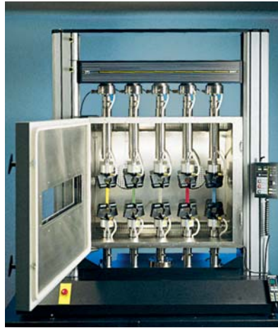
▲ Multiple load strings for high volume test applications
