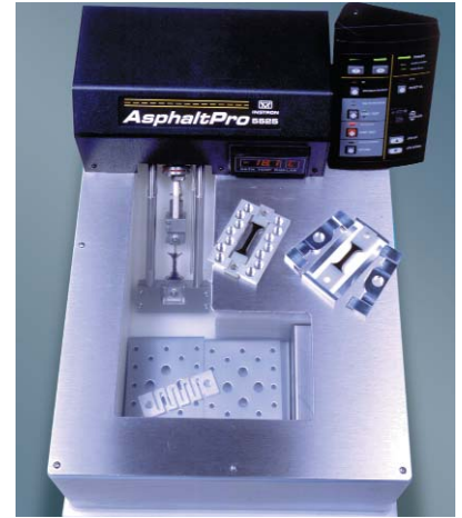
▲ Specially designed frames for asphalt testing applications
